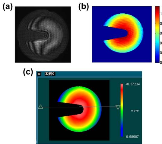
Fig. 6. Comparison experiment results between OCRSI and ZYGO GPI interferometer. (a) Interferogram obtained by OCRSI; (b) and (c) are wavefronts measured by OCRSI and ZYGO GPI, respectively.
