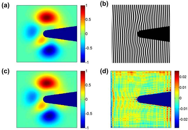
Fig. 5. Simulation results: (a) original wavefront, (b) interferogram with spatial carrier, (c) wavefront retrieved using OCRSI wavefront retrieval method, and (d) residual error between the simulation result and the original wavefront.
