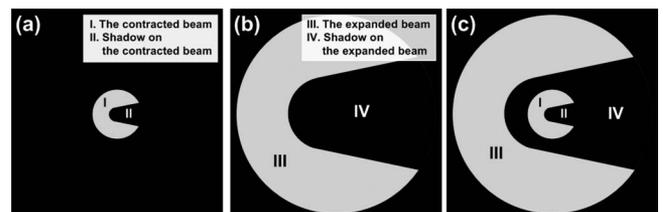
Fig. 1. Schematic diagram of the contracted and expanded beams in the CRSI with model blocking. (a) Contracted beam, (b) expanded beam, and (c) shearogram of these two beams.
