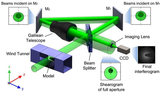
Fig. 2. Optical layout of the OCRSI used for transient hyper-sonic flow field testing.
