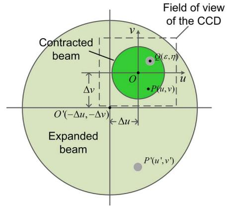
Fig. 4. Schematic diagram of the shearogram in OCRSI.
