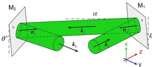
Fig. 3. Schematic diagram of the transmitted beam path reflected by  $M_1$  and  $M_2$  with vertical tilt.
